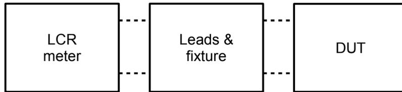
**Figure 18: LCR meter measurement model**
