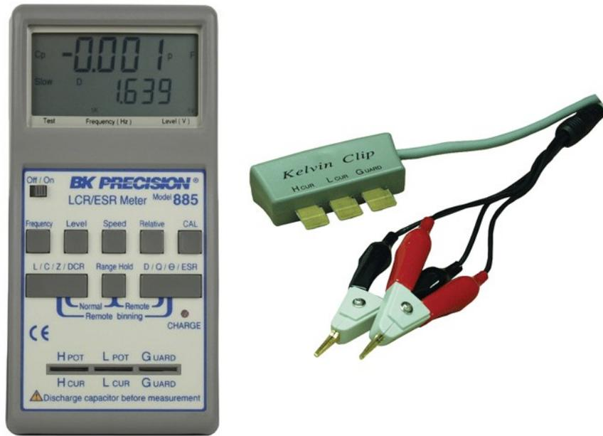
Figure 14: 885 LCR meter with Kelvin clips
